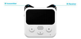
☐ Select the block "send IR message" in the category "Infrared". Have two Codeys send each other different messages. In this way, they detect each other. For instance, two Codeys send messages "red" and "blue "respectively. The messages serve as the bullets.
